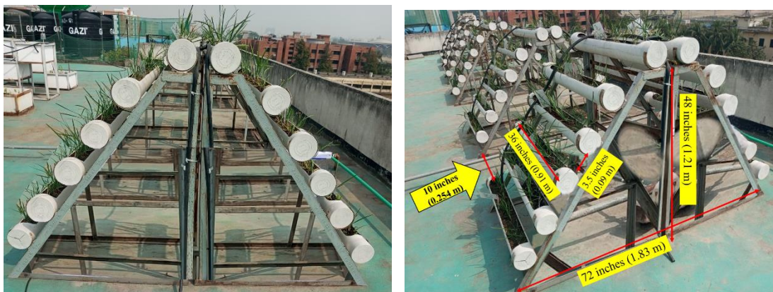
Figure 1. Growth device, structure of vertical garden and a part of the experimental set up.
