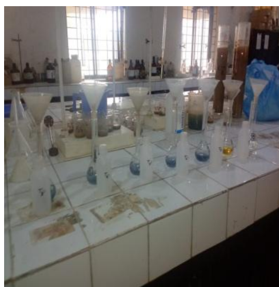
Plate 18: Filtering for determination of Phosphorus (P)
