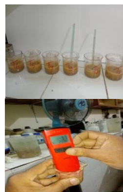
Plate 16: Determination of pH
