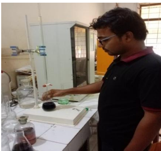
Plate 19: Determination of organic carbon (OC%)
