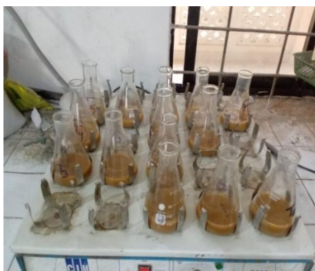
Plate 15: Shaking for determination of Phosphorus (P)
