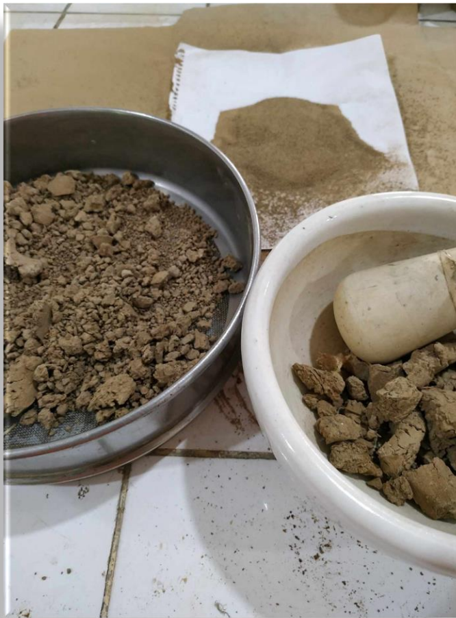
Plate 6. Collecting and processing soil samples for testing
