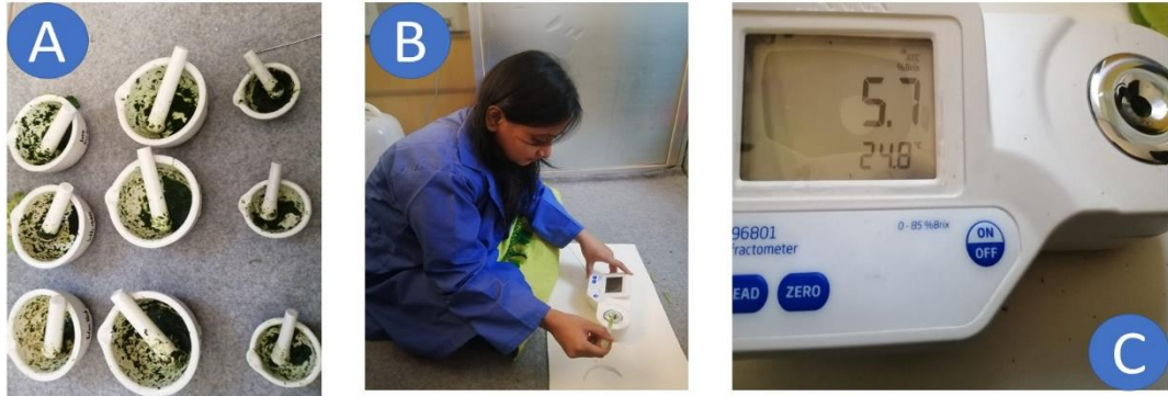
Plate 6: 0 Brix measurement; were A. 9 treatment combination samples B. Operating refractometer for measuring %brix, C. Reading of refractometer %brix
