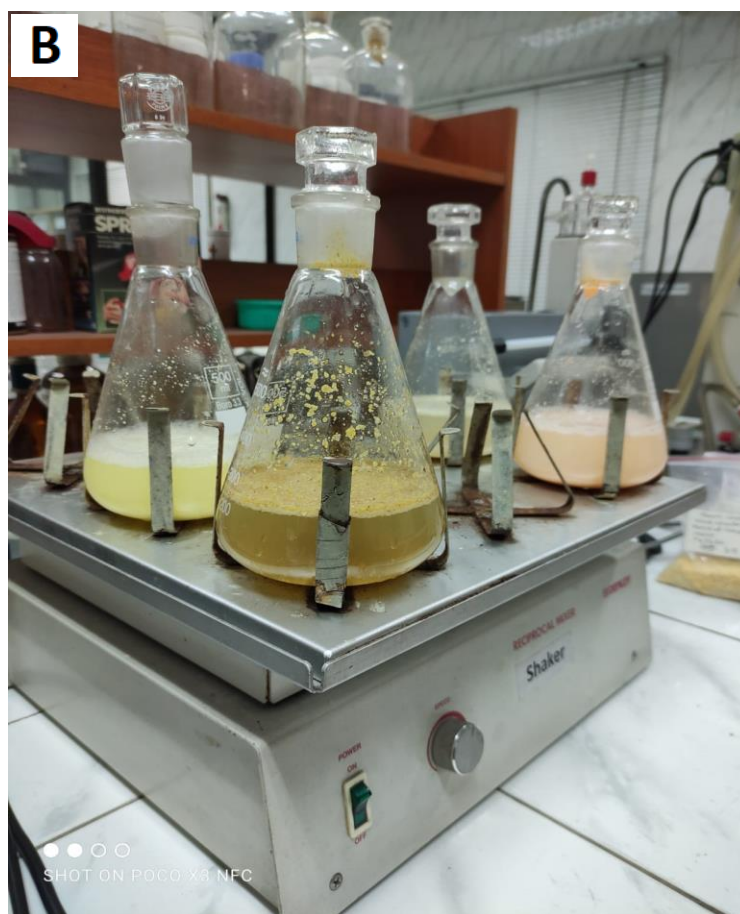
Grinded samples were measured and taken about 25g into a conical flask (A). Shaking into a rotary shaker for the homogeneous slurry formation (B).
