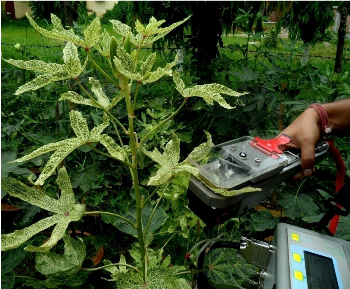
Figure 3: Collection of data over physiological parameters by “LC-Pro + ” machine.
