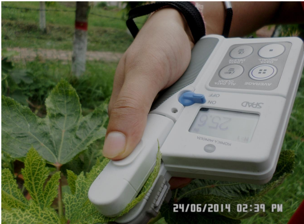
Figure 2: Recording net chlorophyll content in plant leaf by “S-PAD”.
