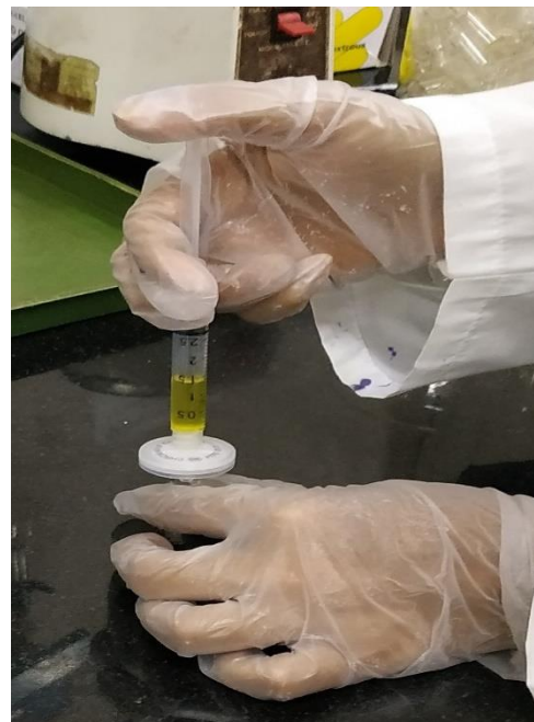
Plate 13. Filtration through PTFE filter
