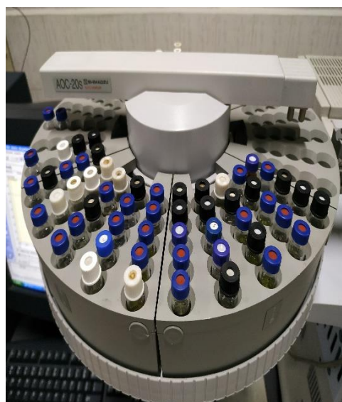
Plate 15. Sample placed in GC for analysis
