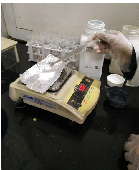
Plate 8. Weighing of salts (NaCl and anhydrous MgSO 4 )
