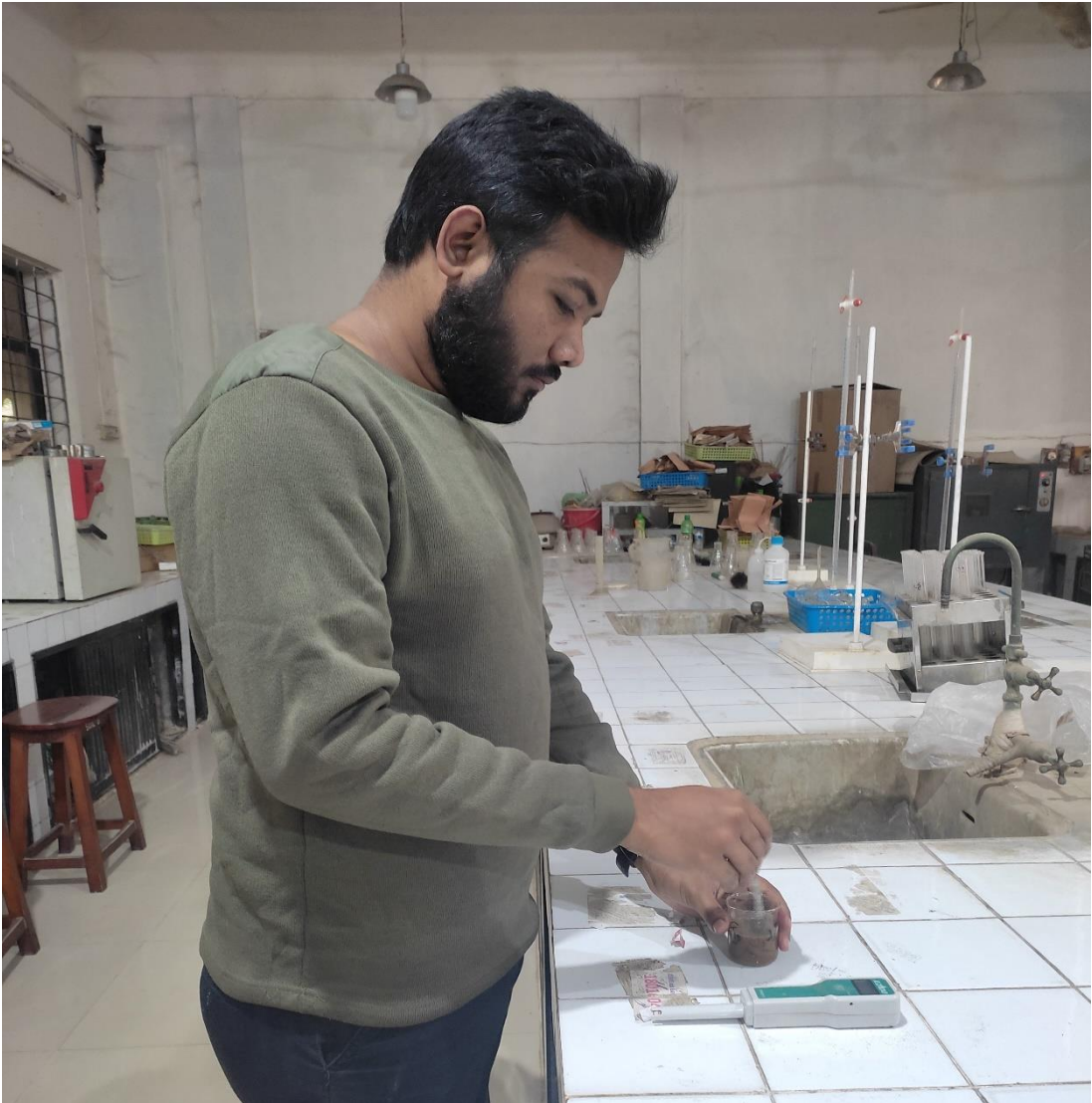
Plate 2: Making soil suspension for pH measurement.
