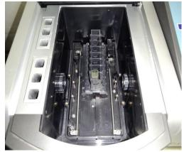
Placement of glasstubes into spectrophotometer
