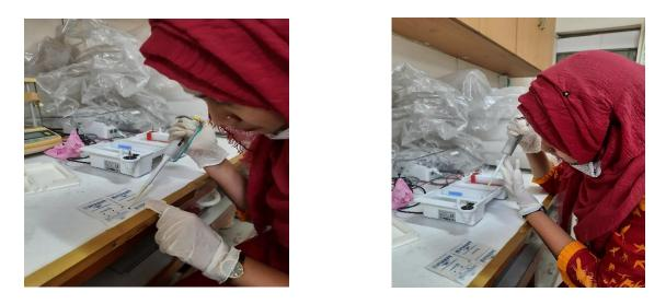
Figure 6. Placement of loading dye with sample into agarose gel
