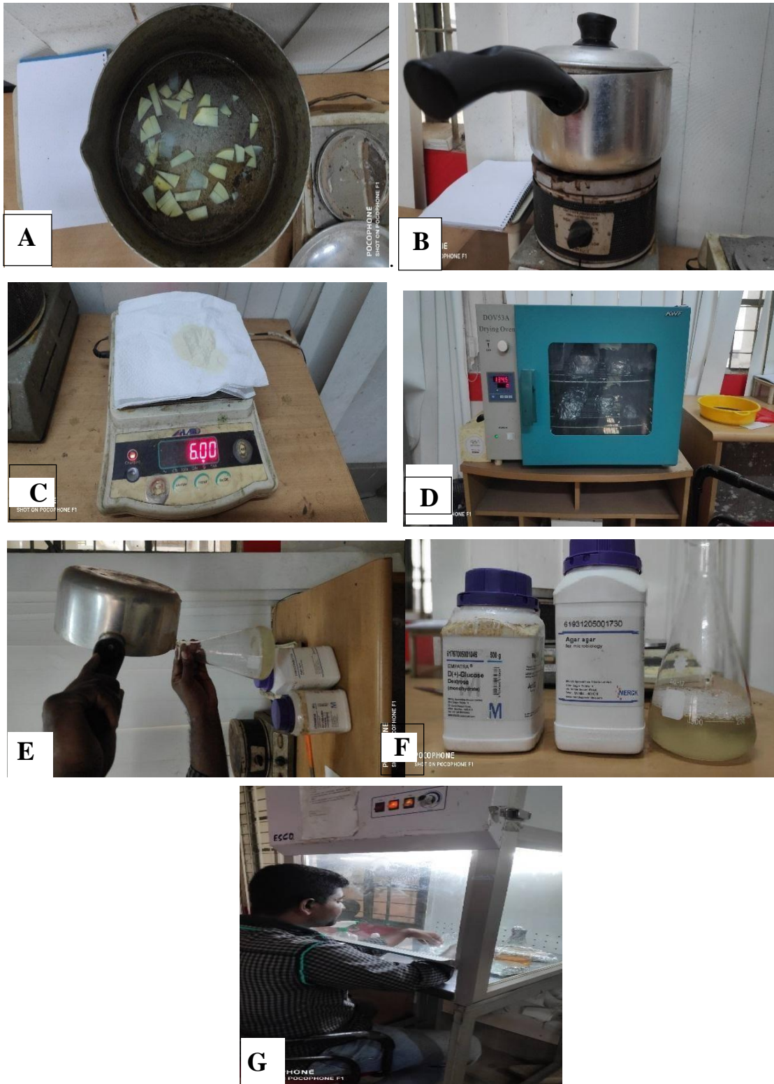
Plate 5. A-B. Boiling of sliced, peeled potatoes (60 g) C. Measurement of weight of Dextrose and Agar (6 g each), D. Sterilization of glassware in oven, E-F. PDA solution (300 ml), G. Prepared PDA solution poured into sterile Petridish
