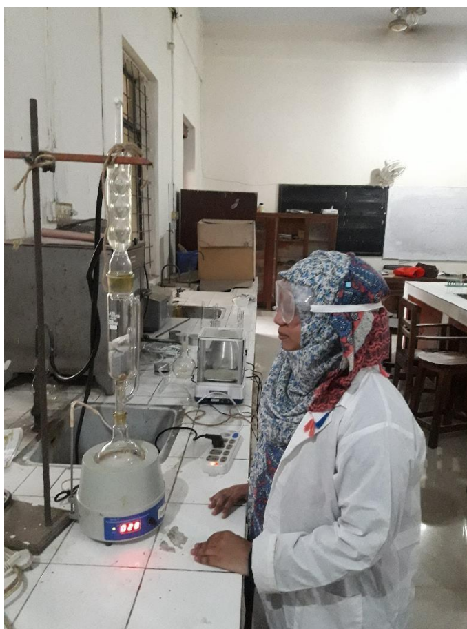
Fig 6: Oil extraction by using soxhlet method.
