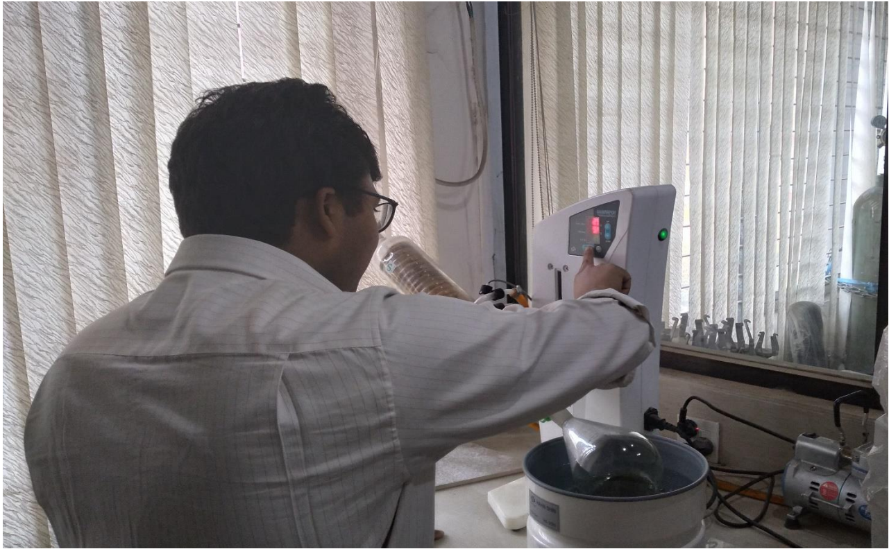
Picture 1: Sample extraction using Rotary Evaporator
