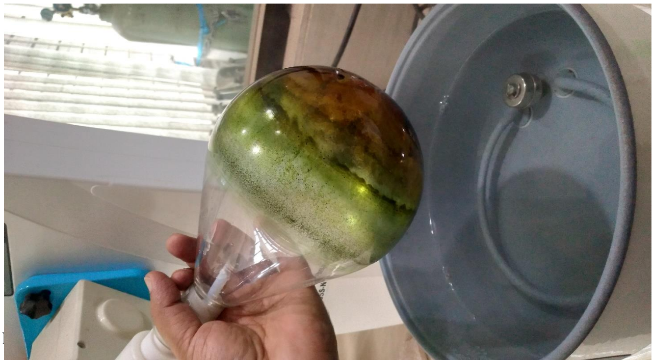
Picture 2: Sample extraction using Rotary Evaporator
