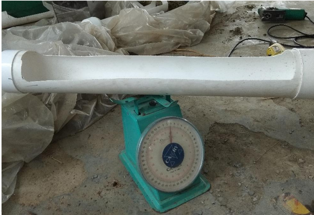
Appendix III. Growth device used in the experiment ( 1 \times 0.1016 \text{ m}^2 PVC pipe)
