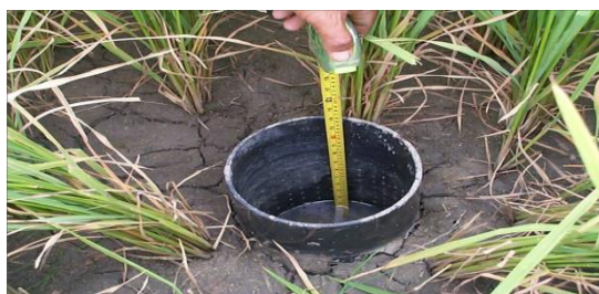
Figure 3.1 Water at 15 cm depth in porous tube
