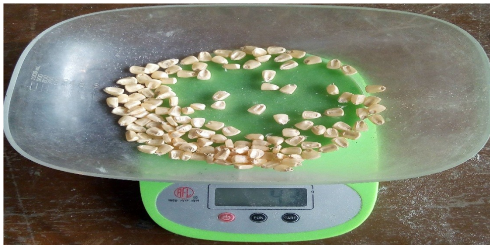
Plate 9. Photograph showing hundred kernel weighing procedure
