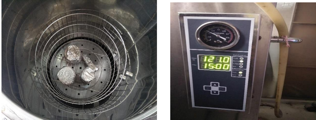
Fig. 1. Sterilization of glass wares by autoclave machine.
