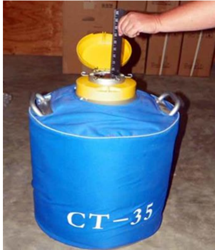
Fig-1: liquid nitrogen tank
