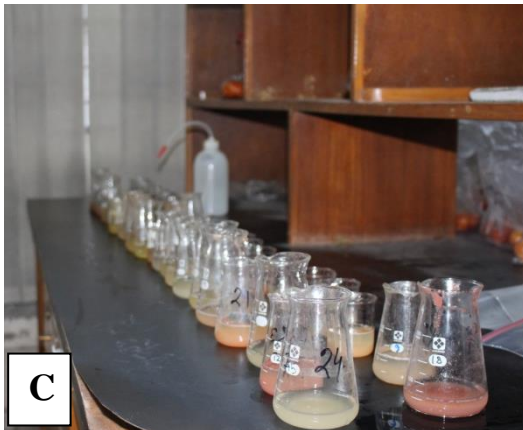
Plate 4. Determination of pH and titrable acidity content A. preparation of tomato juice for pH determination B. Estimation of fruit pH by using REX pH meter model –PHS-3C C. Preparation of fruit juice for titrable acidity determination D. Titration for determination of % titrable acidity.
