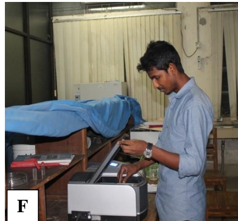
Plate 3. Nutritional analysis in lab A. Determination of Brix% B. Juice of tomato for vitamin C determination C. Titration of tomato juice with dye for vitamin C determination D. Tomato juice with solution on orbital shaker for lycopene content E. development of layer containing lycopene after removing from orbital shaker F. Spectrophotometer reading for lycopene content determination.
