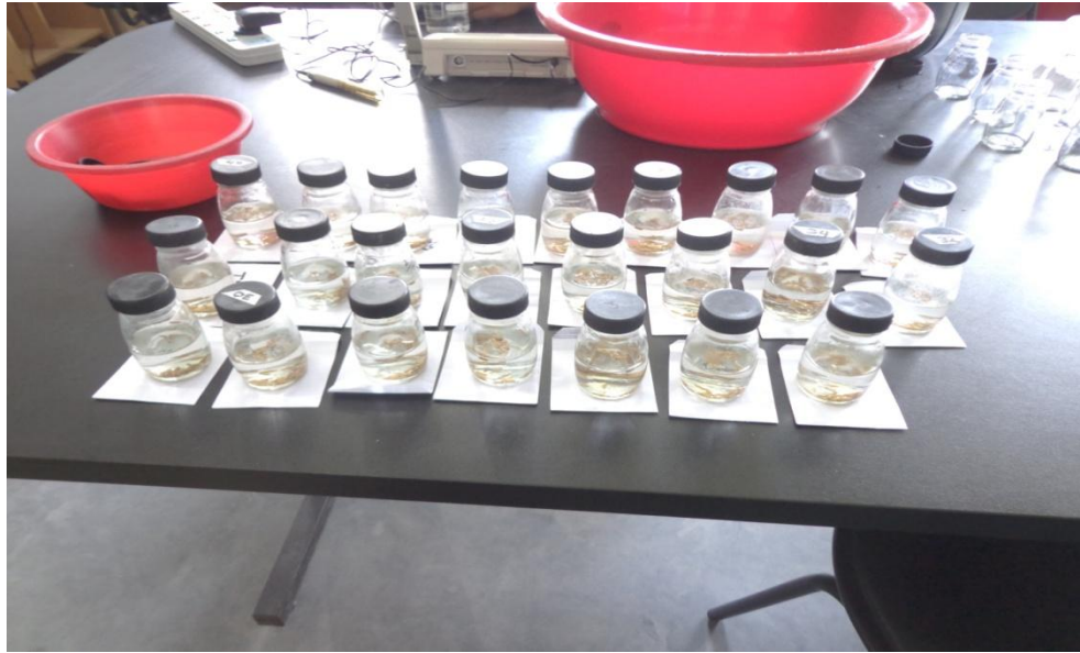
(A) Soaked seed in bottles for electrical conductivity test
