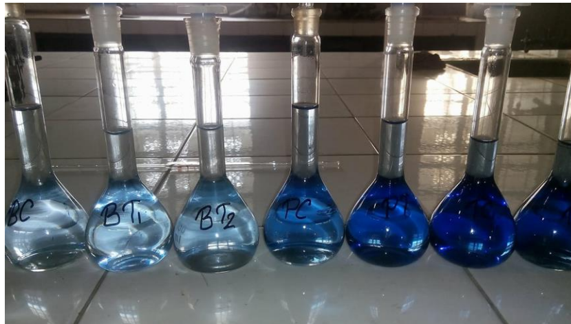
Figure 3.13. Determination of Phosphorus in fruits and vegetables
