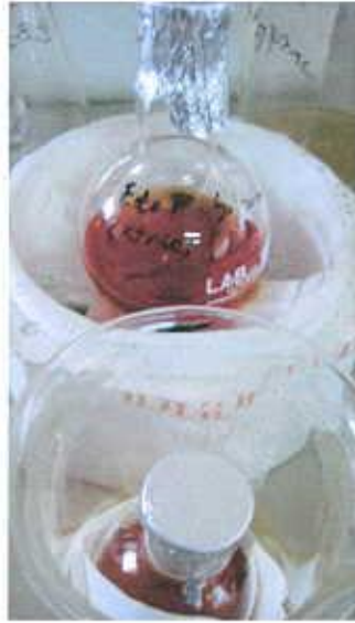
Plate 11. Concentrated sample after evaporating
