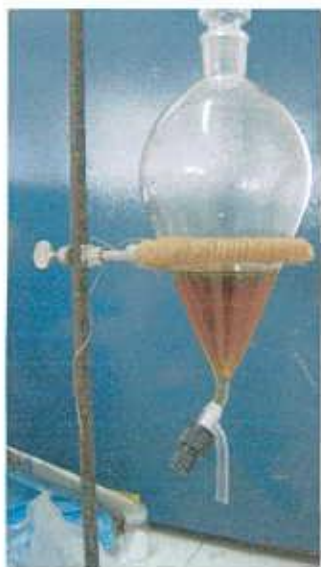
Plate 9. Separating of the organic part by separating funnel
