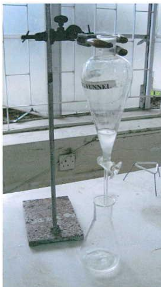
Plate 13. Separating organic part with a separating funnel
