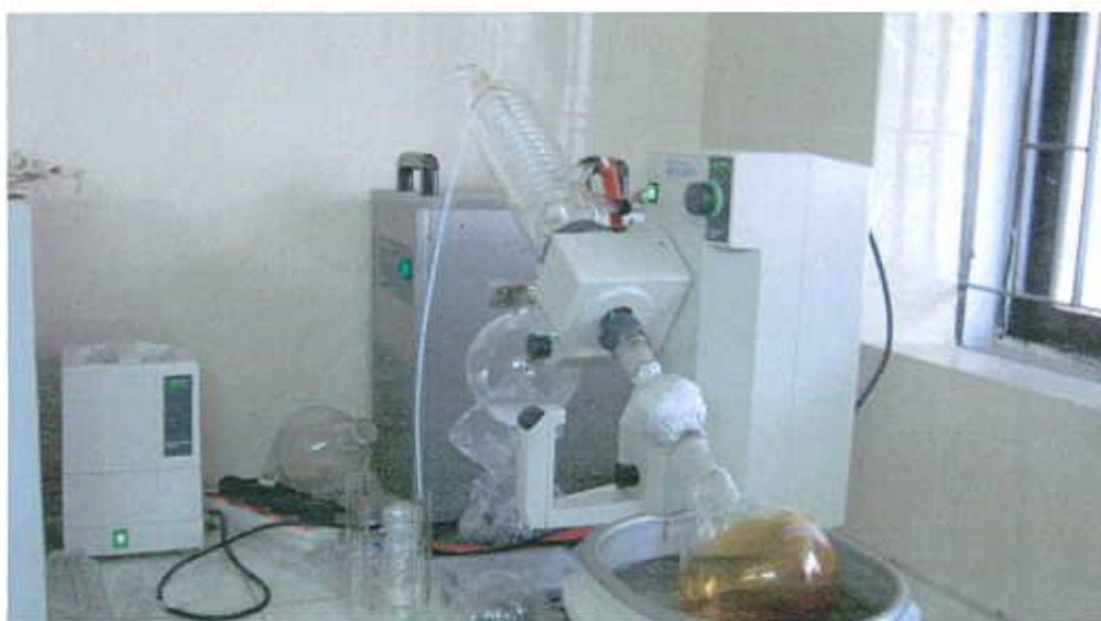
Plate 10. Evaporation by rotary evaporator
