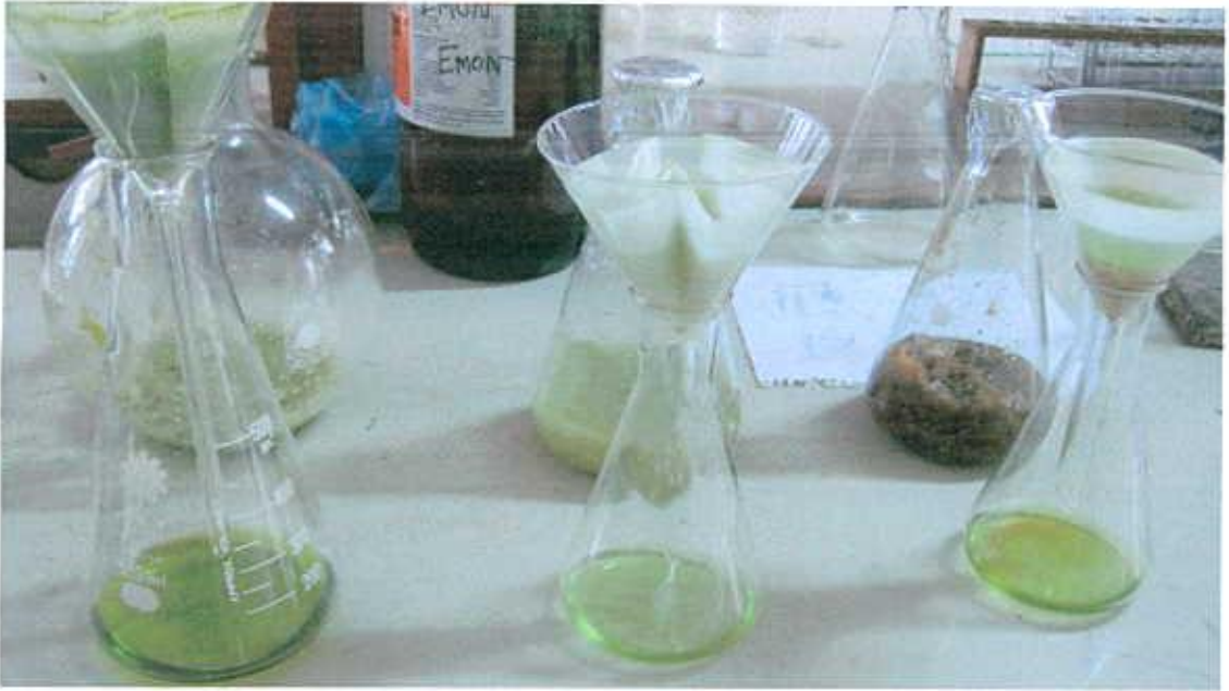
Plate 7. Filtration of the blended sample for extract preparation
