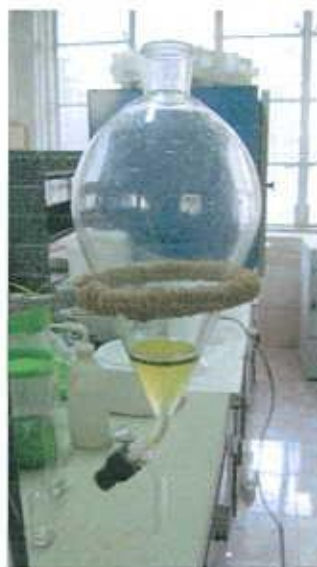
Plate 9. Separating of the organic part by separating funnel
