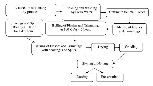
Fig. 1. Schematic Diagram of Vegetable tanning by-product Preparation
