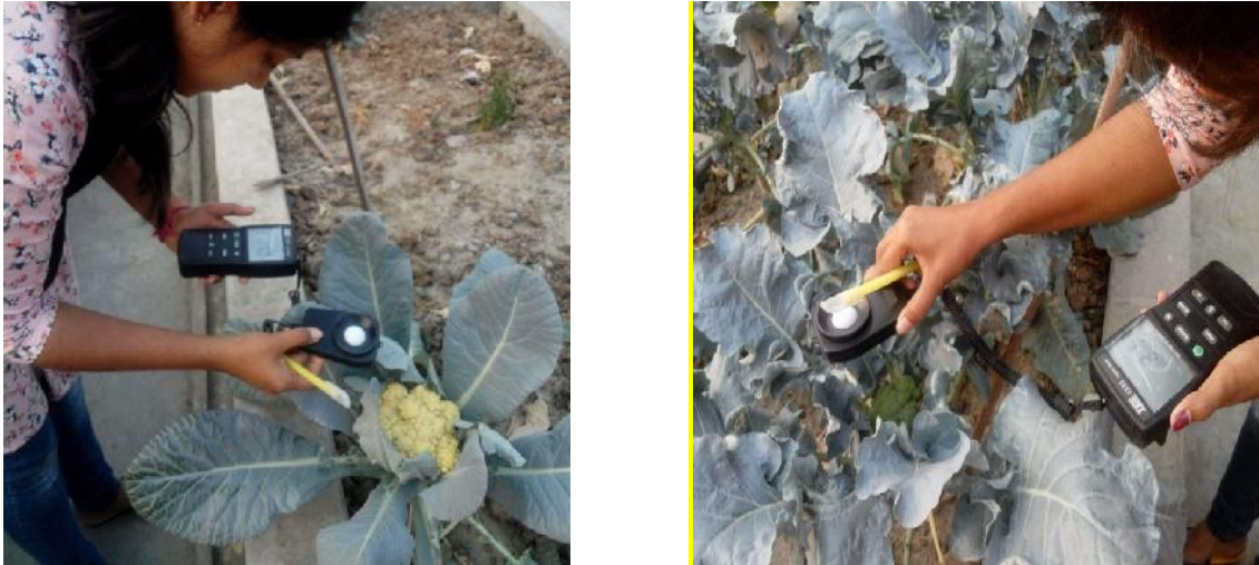
Plate 8: Measuring the light intensity in experimental crops.
