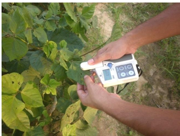
Figure 3. Recording net chlorophyll content in plant leaf by “S-PAD” meter
