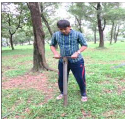
Plate 5. Inserting Auger in the soil
