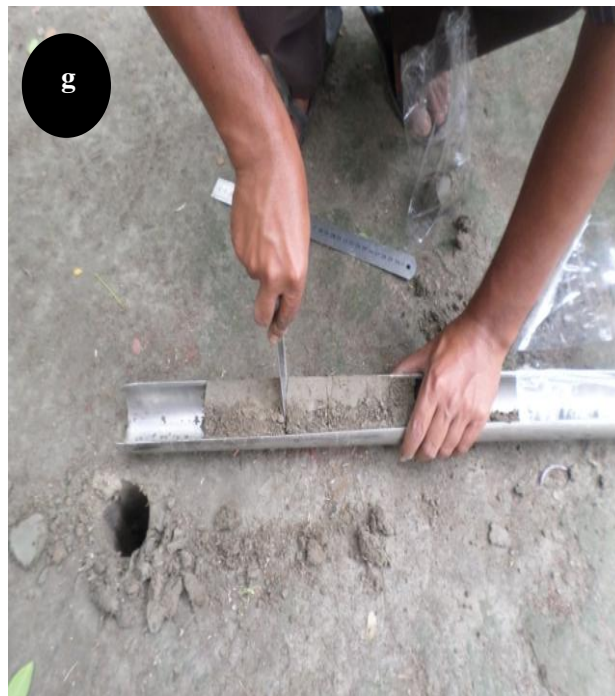
Plate 3: Photograph shows (e) measurement of GBH (f) inserting auger into the soil and (g) Carefully taken the soil sample.
