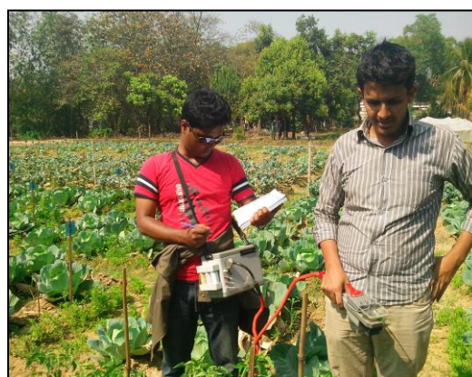
Photograph showing, data collection with LCpro+ Meter for measuring carbon assimilation rate.
