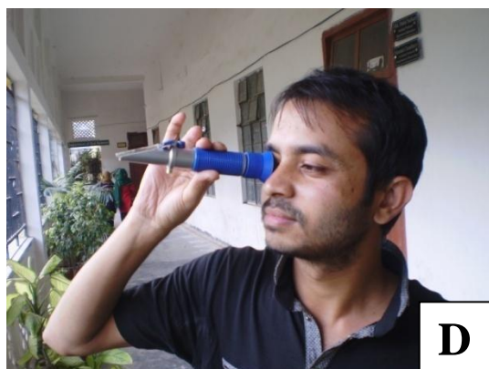
Plate 3. Different types of activities for data recording. A. Extraction of lycopene and B. Shaking for extraction of Vitamin-C. C. Solution preparation for extraction of vitamin-C D. Estimation of brix (%) using Portable Refractometer
