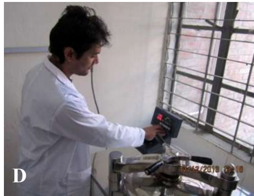
Plate 1. Steps of media preparation. A) Sterilization of glasswares, B) Preparation of medium solution, C) Adjustment of pH, D) Medium sterilization and E) Aliquot under laminar hood
